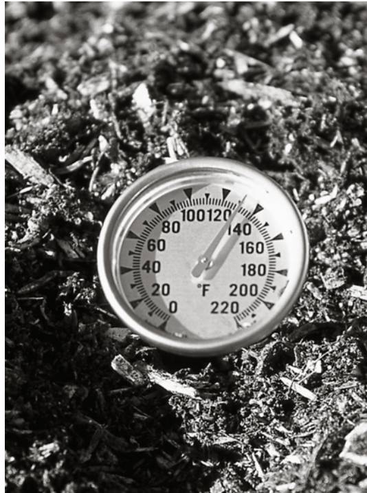
Figure 11. Effective composting takes place at temperatures of 55 to 65°C (130 to 150°F).
